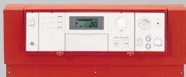
Digital outdoor reset boiler control for modulating burner, boiler water temperature and up to two heating circuits with mixing valves. Domestic hot water heating is a standard feature with this control.
