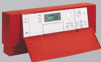
Digital outdoor reset cascade control for up to four heating boilers. Designed to operate with or without setpoint demands from BMS or DDC systems. The Vitocontrol-S will modulate burners, stage and rotate boilers, regulate boiler water temperature, common supply temperature and up to two heating circuits with mixing valves. Domestic hot water heating is a standard feature with this control.
