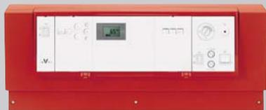
Digital boiler setpoint control designed for external demands from BMS and DDC systems using a 0-10 VDC or LON signal or for maintaining constant boiler water temperature without demands. Provides easy single cable connection to the Vitocontrol-S for multiple boiler application. Domestic hot water heating is a standard feature with this control.
